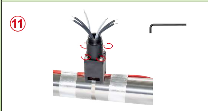
11: Compress the seal by screwing the upper part of the foot with the 4 screws until the both parts are in touch
